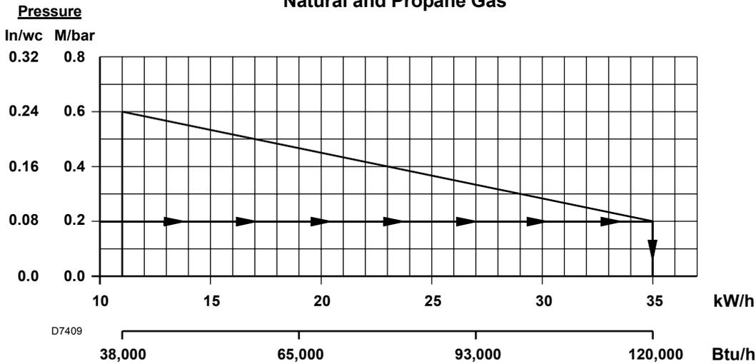
Any change from zero (0) pressure in the combustion zone will affect the Btu output of the burner. To supply the required input to the appliance, manifold pressure will have to be adjusted to compensate for this condition.
