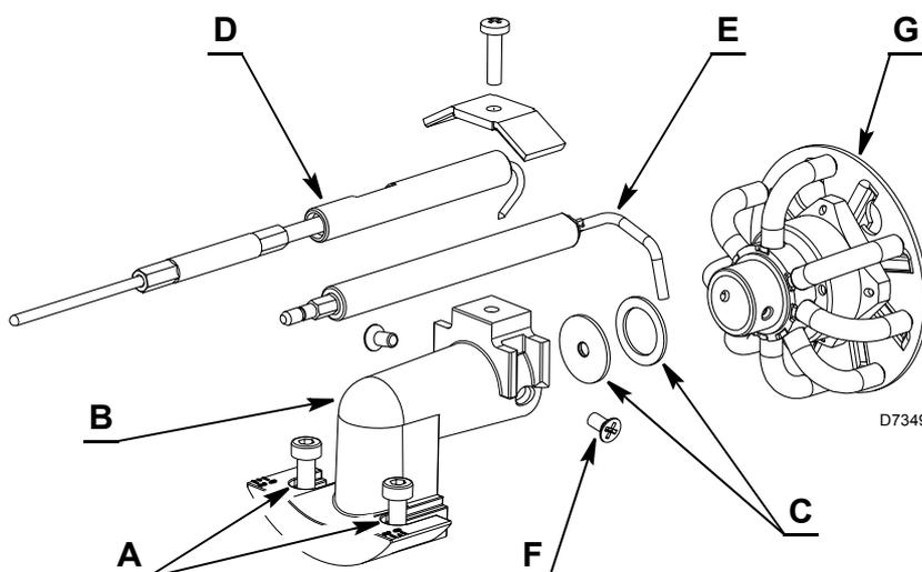
Slide the elbow (B) so that the number on the indicator scale aligns with the back edge of the air tube.
